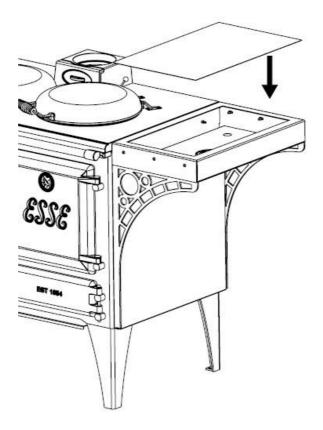
.The unit is supplied with a stainless steel panel for fitting when the unit is to be a Hostess shelf. The panel has double sided tap applied to the rear. Peel off the tapes protective strip and fit the shelf paying attention to insure the panel is central and level. Press down on the edges of the panel to ensure good adhesion. The stainless steels protective film can now be removed.
