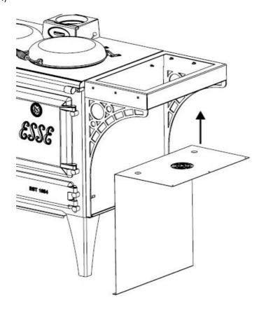
Using a pozi-head screw driver fit the bottom cover plate with the 5 self tapping screws supplied.
