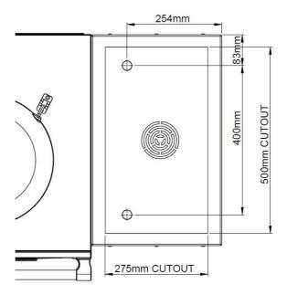
If you would like to install a domino hob, this is the stage that you would do this. The cut -out size in the shelf is 275mm x 500mm. There are knock panels in the bottom cover plate to allow cables or pipework. Use the grommet supplied in the knock outs when running cables or pipework. Use the instructions supplied with your chosen domino hob for installation information.
