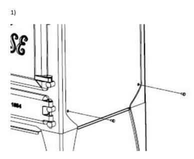
Using a 10mm spanner remove the two screws located on the side panel of the cooker (Right hand installation shown). Keep these screws safe.
