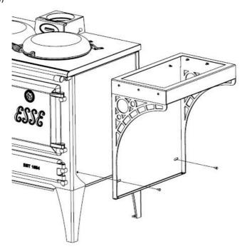
Hook the Hostess Shelf Frame over the top of the side panel (in the gap between the cooker top and the side panel) and align so the back of the shelf is level with the back of the cooker top.
